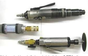
It is important to note that most air tools have 2 CFM ratings: Under no load (free moving) and Under load (doing work)
