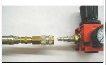
Connect the air tool used most often at the air drop location.
