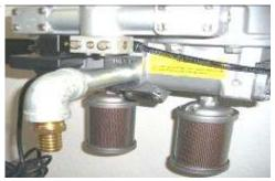
Assemble the nipple and union then install on the outlet port of the SFD Dryer
