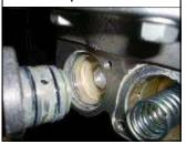
Step 2 Remove unloading purge valve.
